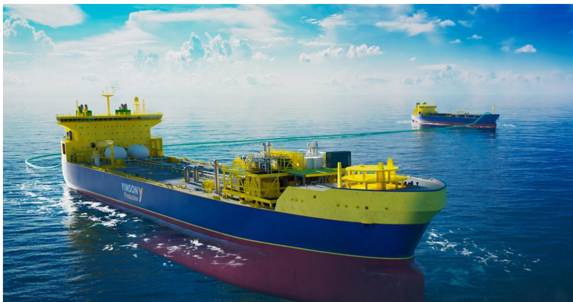
An illustration of an FSIU (in the foreground) receiving cargo from a LCO 2 carrier (in the background).
